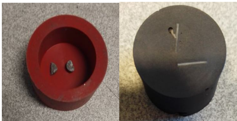
Figure 12. Mounting of samples using cold resin.
