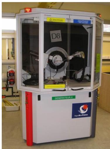
Figure 2. 11. diffraction de rayons X BRUKER AXS D8 ADVANCE
