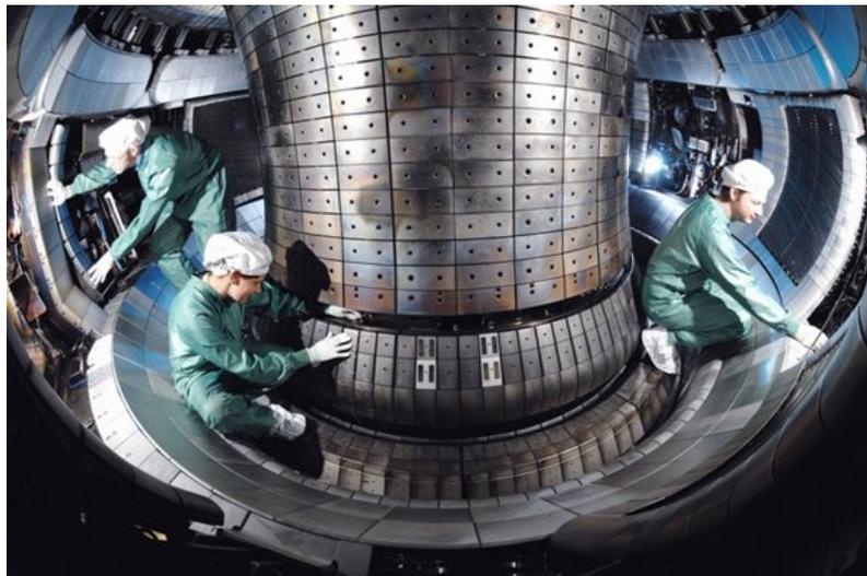
Figure 2.1 – Interior view of the ASDEX Upgrade tokamak during installation of the tungsten plasma facing components (source: IPP web-page).
