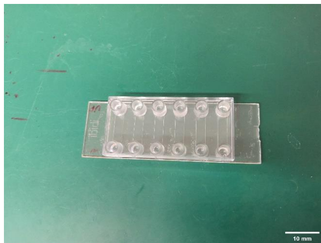
Figure 2-3 Finished glass-bottom flow chamber device containing six 17mm x 3.8 mm x 0.4 mm channels
