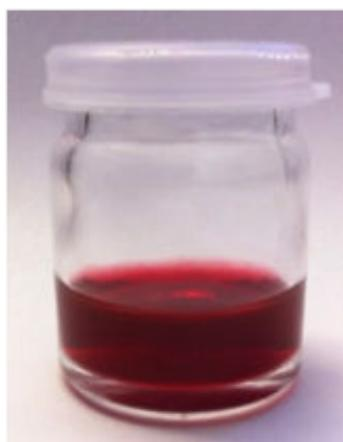
Figure 2.15: A photo of gold nanoparticles solution obtained by the ablation of a bulk target in aqueous PEG solution.
