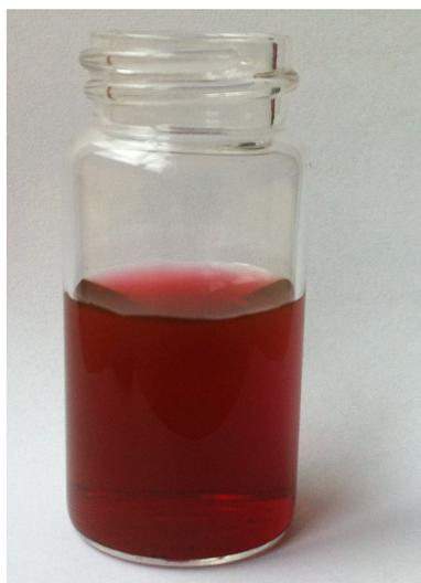
Figure 2.7: Colloidal solution of the gold nanoparticles obtained after the ablation from a bulk target.
