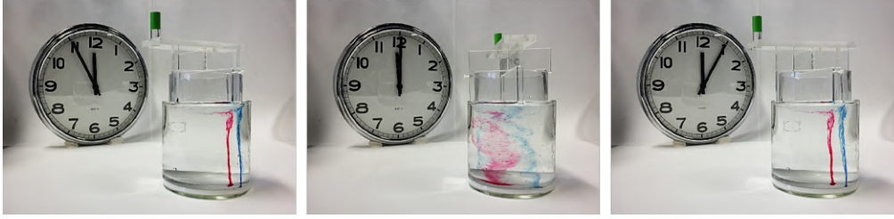
Figure 2.6: Time reversibility of Stokes. Fluid has been injected between two concentric cylinders, with dyes injected inside the fluid. One of the cylinders is then slowly rotated to be in the Stokes regime, which smears the dye, making it appear mixed. The rotation is then reversed, and we recover the same initial pattern, highlighting the reversibility of Stokes flow [191].
