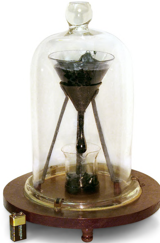
Figure 2.1: Picture of the pitch-drop experiment, highlighting how pitch, despite looking like a solid, flows like a fluid over long time scales [154].
