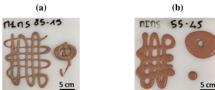
Figure 28 : (a) KM1_{50}M5_{50} extrudable et (b) KM1_{50}M5_{50} non extrudable.
