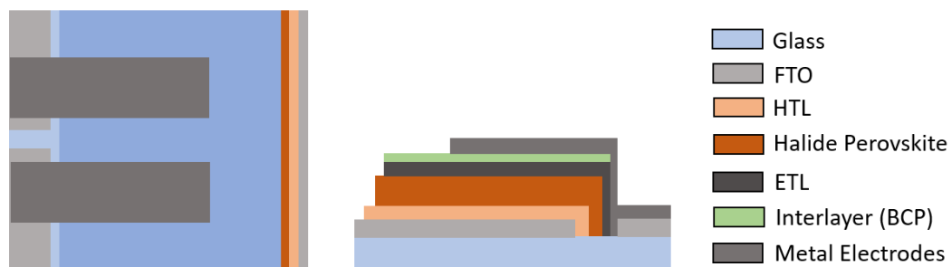
Figure IV.29 : The design of metal electrodes on the ETL
