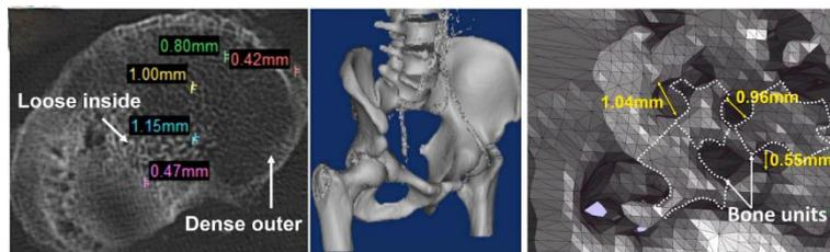
Fig 1.1 The design process for complex bio-inspired unit cells<sup>39</sup>
