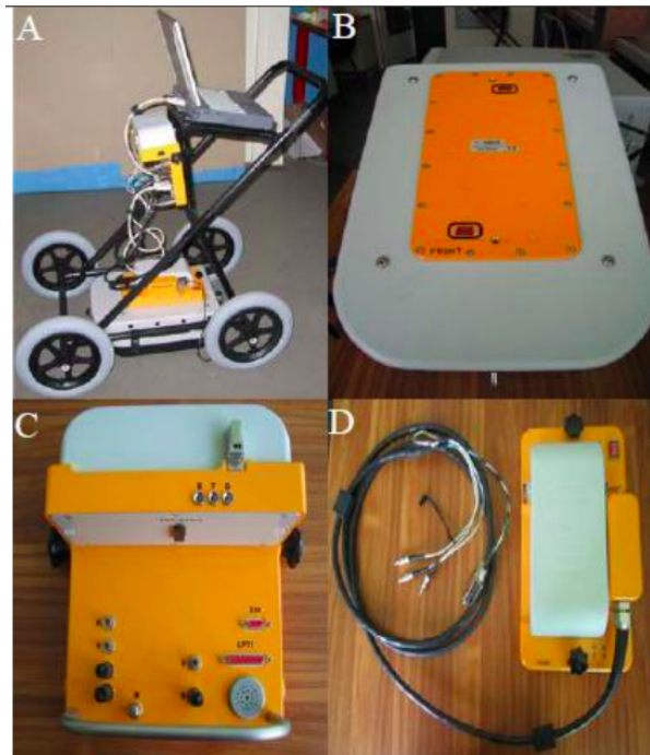
Figure 4.4: Radar GPR RAMAC
