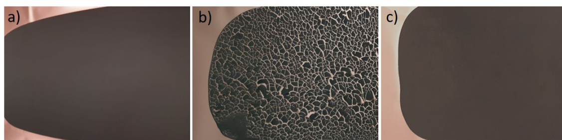
Figure 4.6: Photographs of tape casted anodes with different compositions: a) Si \Omega C as active material, PEDOT:PSS as binder, b) Si \Omega C as active material, CMC of M_w 90 000 as binder, c) Si \Omega C as active material, CMC of M_w 90 000 as binder + 9wt% of latex Duramax B-1000.
