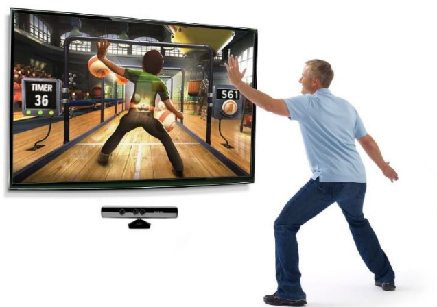
Figure 2: Microsoft introduced Kinect sensors for gaming purposes with the Xbox console. The sensor can track human body and hand motion without the use of any controller. (Image from [URL9])
