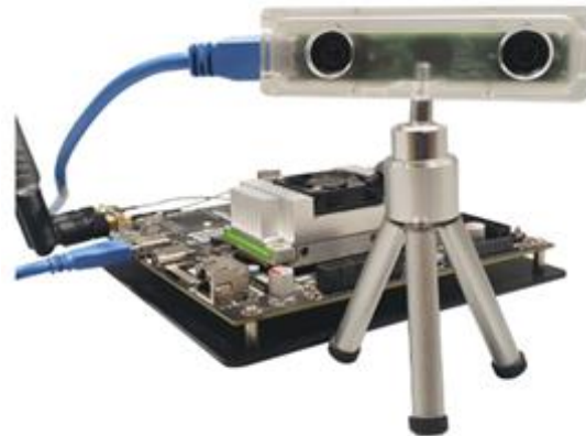
Figure 4: TaraXL camera from e-con Systems™ [URL7] uses passive stereo technique to capture the depth. It uses two lenses to capture images of a scene from different viewpoints, and then uses the triangulation method to calculate the depth.
