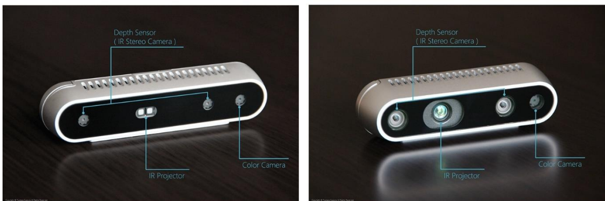
Figure 6 : Intel Realsense D415 (left) and D435 (right). They both use stereo vision with an infrared projector. Figure from [URL2]
