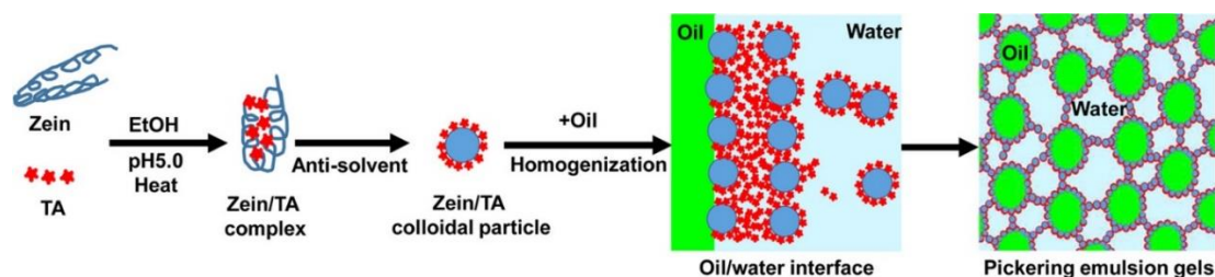
Figure 12. Schematic illustration of the preparation of emulsions gels stabilized with zein/tannic acid complex colloidal particles. The synthesis of zein/TA complex is performed at pH 5.0, then zein particles are coated by TA via an antisolvent method to form zein/TA colloidal particles. These particles are then used to form Pickering emulsion gels. (Ref 123 with permission from the American Chemical Society)
