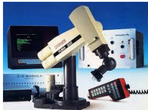
(d) PUMA (Programmable Universal Machine for Assembly) robot by Unimation (1978)
