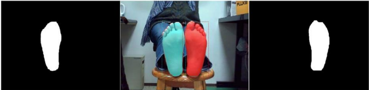
Figure 29: Segmentation con R-CNN and the generated masks in visible spectrum images. The database for training is a set of 300 images [75].
