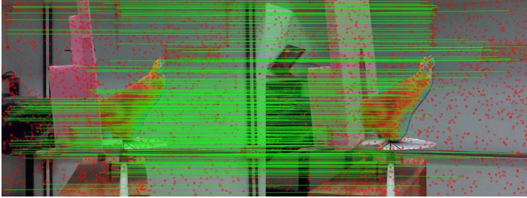
Figure 86. Detected feature points (red dots) and their correspondence visualized (the green lines represent the link between homologous points). This graph shows 202 matches between images 6 and 7 from set S1, with most of the critical points discarded, demonstrating that the model's quality is dependent on the precision of the matching points procedure.
