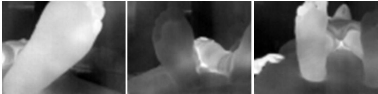
Figure 18: Images taken with the Lepton 2.5 sensor which have not been calibrated. These images were generated by reconstructing raw information recorded through digital processing. The RoIs (i.e. de plantar foot) are eclipsed by other regions, such as the volunteer body or surrounding people, with higher intensity in all three cases. The temperature interferences due to wrong data or image acquisition may challenge data processing from the perspective of a quantitative point of view. The images were taken from [67].
