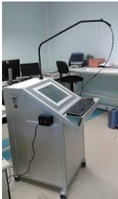
Figure 1.19: SpectroLive device in the operating room (left) and clinical measurement protocol (right).
