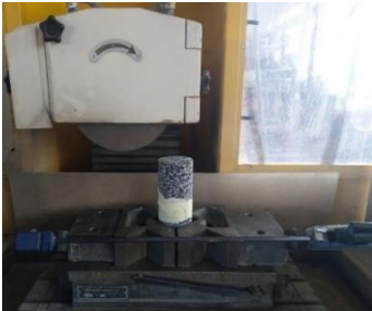
Figure II-16. Sample Surfaces' polishing
