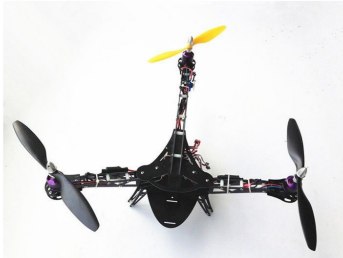
FIGURE 1.4 – Exemple de drone tri-rotor
