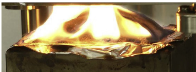
Figure 1.11: Intumescent coating formed from intumescent-based polypropylene after ignition. Ammonium polyphosphate is used as an acid source and tris(hydroxyethyl) isocyanurate (THEIC) as char former. Taken from Bourbigot et al. 2019 [63].
