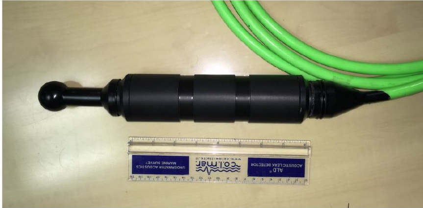
Figure 2.7: Picture of a Colmar hydrophone.
