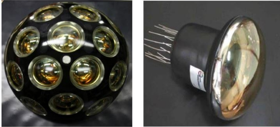
Figure 2.3: A Digital Optical Module (left) and a photomultiplier (right).
