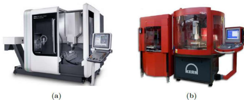
Figure 2.26: (a) CNC 5 axis milling center: DECKEL MAHO, (b) CNC 5 axis micro milling center: KERN EVO.
