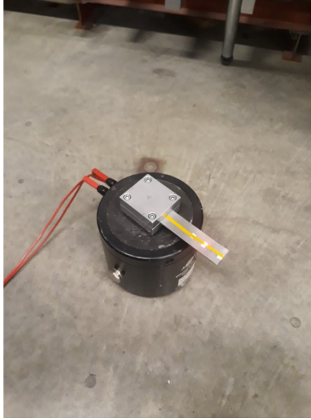
Figure 5.8: Experimental setup for the aluminum beam with a constrained viscoelastic layer
