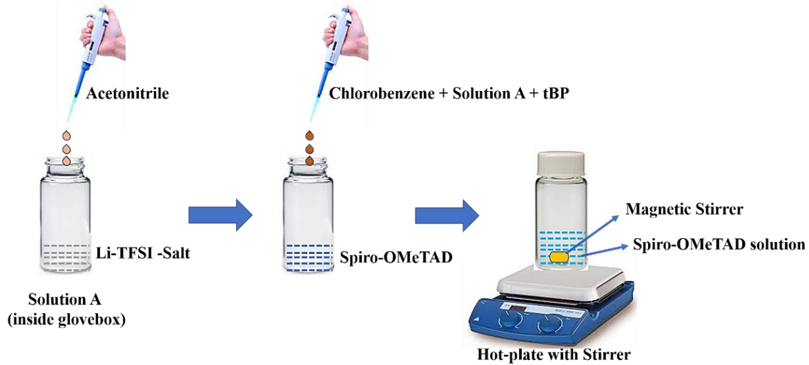
Fig. 3.4. Schematic of HTL solution preparation procedures.
