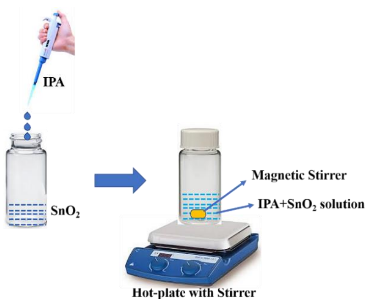
Fig. 3.2. Schematic of ETL solution preparation procedures.
