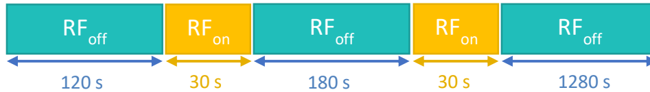
Figure 106 : Schema of the time slots assigned to the RF exposure and to the no RF used with the microfluidic channel.
