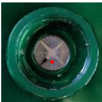
Figure 71 : Fluorescence recorded at the lower section of the MEA-1, a) photo of MEA-1 with red dot representing the position where the fluorescence intensity and temperature were recorded, b) image recorded by the microscope 20x objective of the MEA-1 showing the lower conductor lines.
