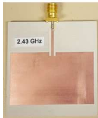
Figure 13 : A microstrip patch antenna operating at 2.43 GHz [86].
