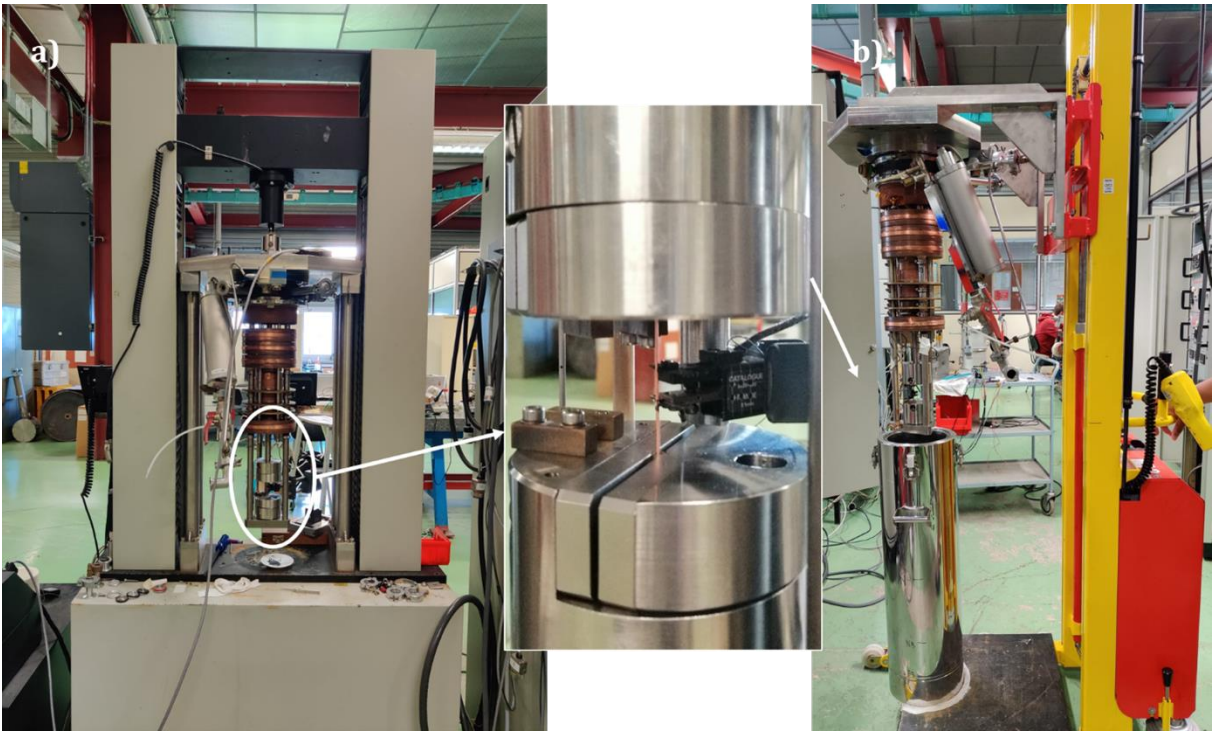
Figure II.2.7. a) INSTRON 5500R tensile machine for cryogenic tests; b) insertion of the device with clamps, sample and extensometer into the cryostat.
