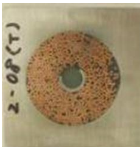
Figure IV.2.11. Destructive examination of LTP CS conductors after cycling: visible displacement of the wires (Hemmi 2012).
