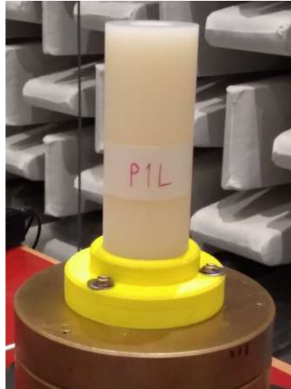
Figure 1.21: Tube P1L placed on the sensor impedance for measurement.
