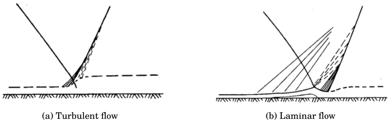
Figure 1.9: Reflected shock pattern. From [102].
