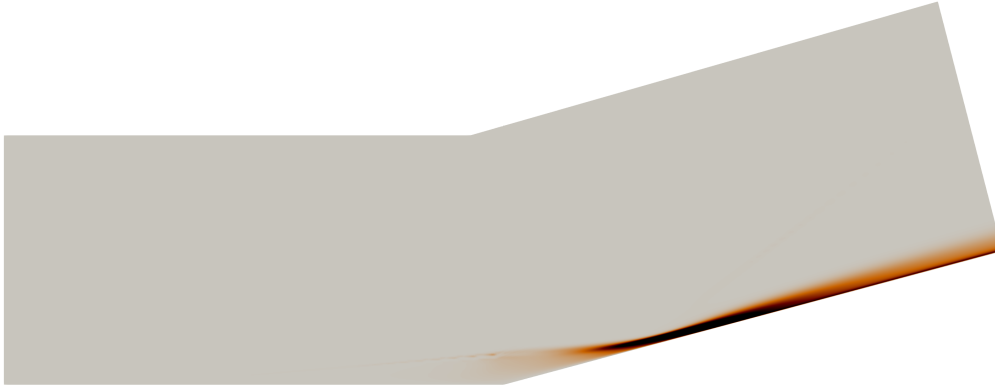
Figure 5.13: SingleRamp: Time- and spanwise-averaged turbulent kinetic energy field.
