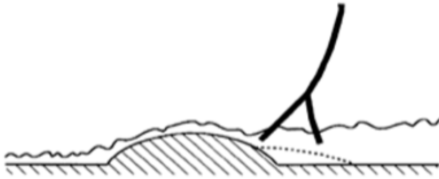
Figure 1.5: Transonic flow over a bump. From [96].
