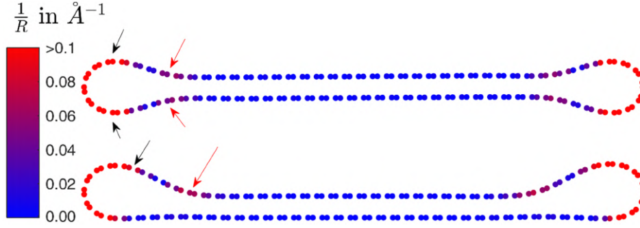
Figure 4.16: Curvature of collapsed carbon nanotube (top) before and (bottom) after substrate-induced deformation. The borderline of hybridization change between flat middle section and folded edges is indicated by red arrows. In this section it is expected a change of electrostatic potential, which induces the electron back-scattering process necessary to activate the D band. The highest point of edge cavities are indicated by black arrows. Image taken from Paper III. Credit: Pascal Puech.
