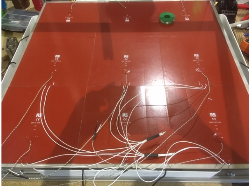
Figure 5.4: Photography of the heating silicone plates attached to the bottom of the stainless steel plate. The central plate is linked to a power supply and the 8 others to another power supply, in order to control the central plate individually.
