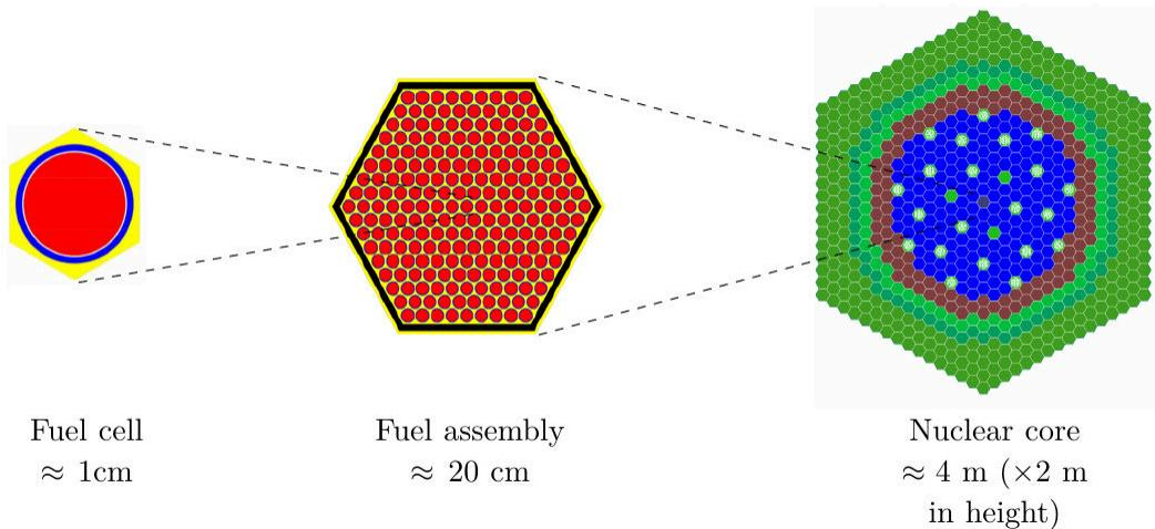
Figure 1.3 – Typical SFR geometries and dimensions
