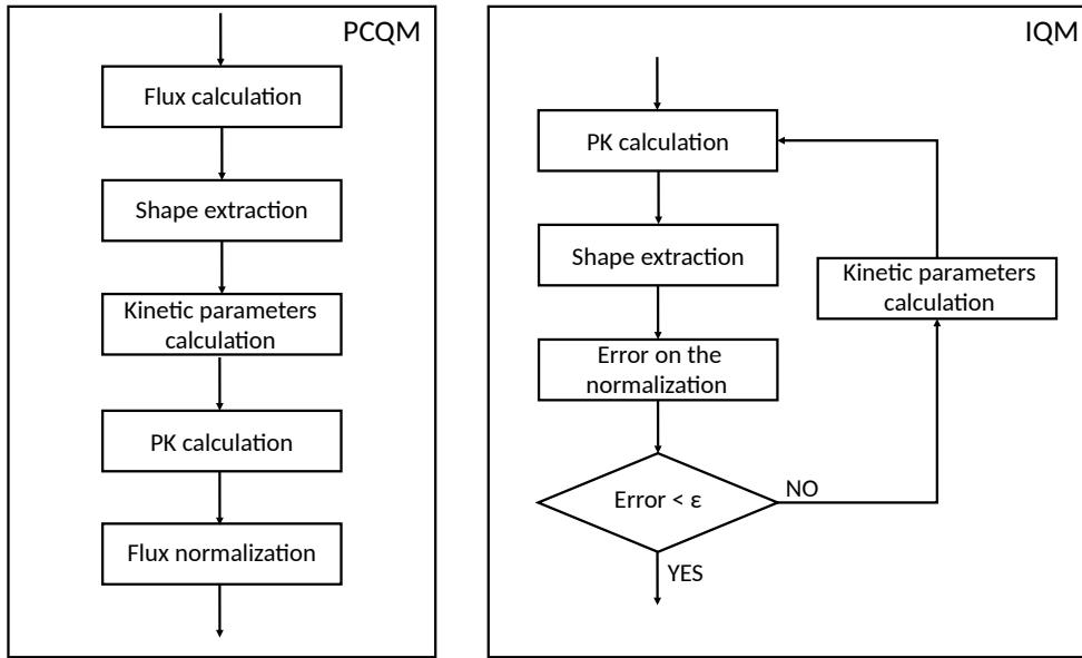
Figure 3.2 – Flow chart of the two methods
