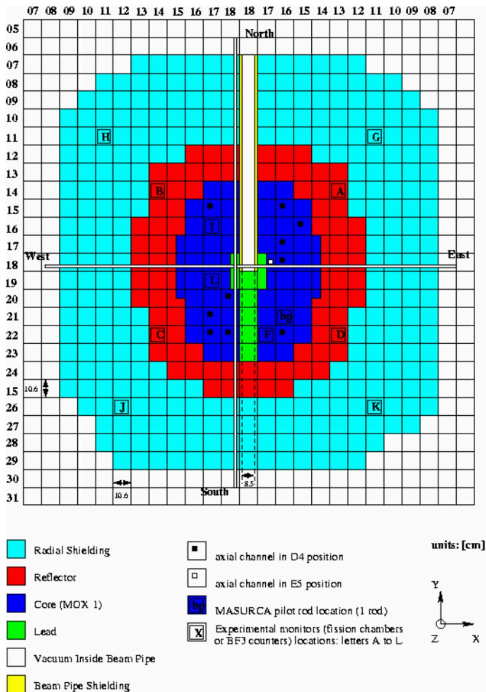
Figure 5.11 – Horizontal section of the experimental configuration - MUSE
