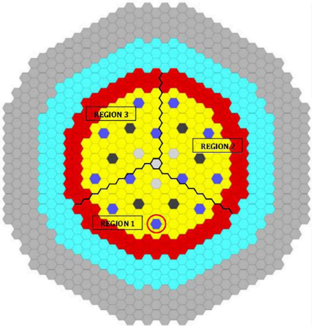
Figure 5.1 – ASTRID CFV-V1 - Color code: Yellow: inner fuel - Red: outer fuel - Light blue: reflector - Grey: shielding - Dark blue and black: control rods - White: inert sub-assemblies
