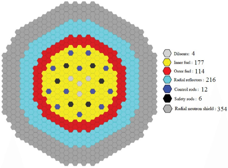
Figure 4.1 – ASTRID CFV V1 core
