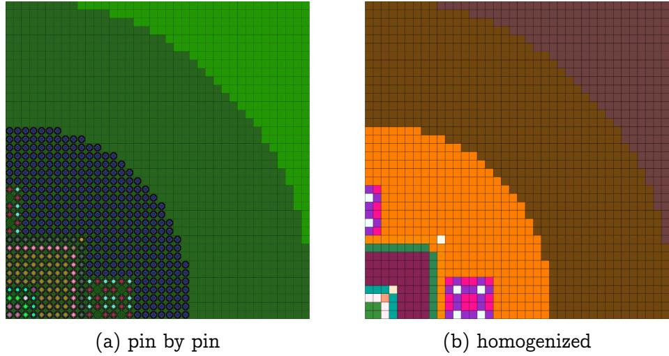
Figure 4.3 – IDT 2D geometries modeling
