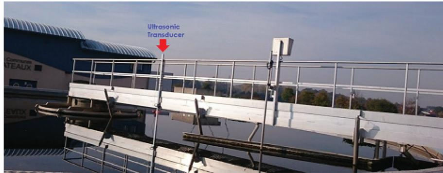
FIGURE 4.6: Overview of the support and Peacock UVP system placed in the clarifier
