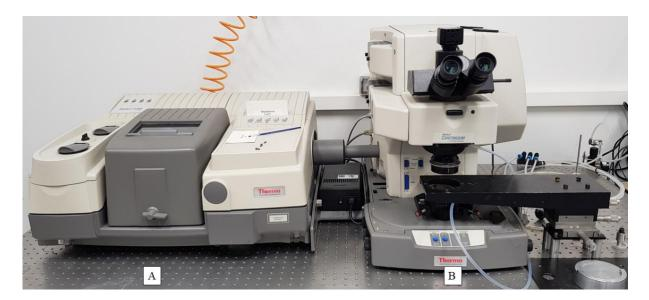
Fig.I.7: A) Nicolet FTIR 5700 spectrometer at LPG; B) IR microscope equipped with the X15 Cassegrain objective
