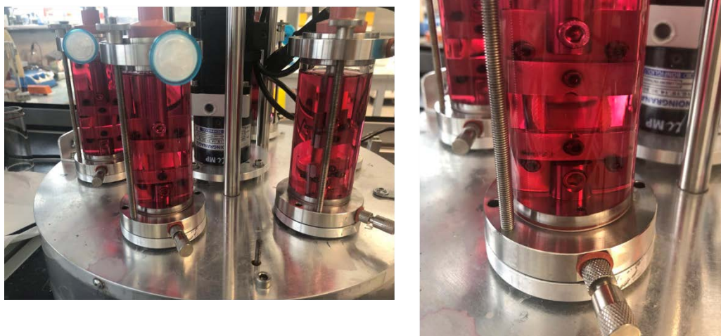
Figure 10 The tension-torsion bioreactor designed by our team.
