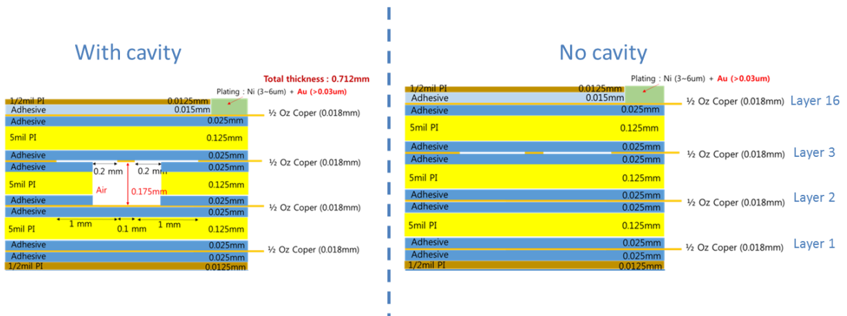
Figure 2.26 The stack up of the low cost antenna array with and without the air cavity
