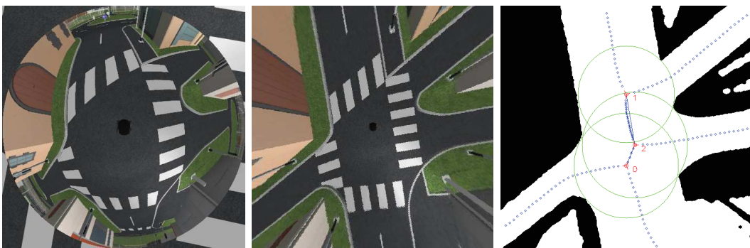
1) Image omnidirectionnelle 2) Bird-eye view 3) Carte hybride locale
