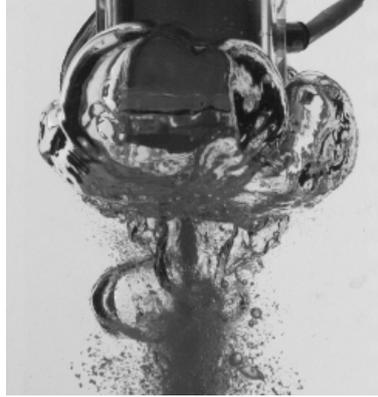
Figure 6.12: Snapshot of the discharge of a silo immersed in water with an instantaneous rupture of the outlet for  $L = 40\text{mm}$ ,  $D = 10\text{mm}$ ,  $d_p = 180\mu\text{m}$  (hydrophobic ceramic particles) and  $h_{\text{water}} \approx 80\text{mm}$ .
