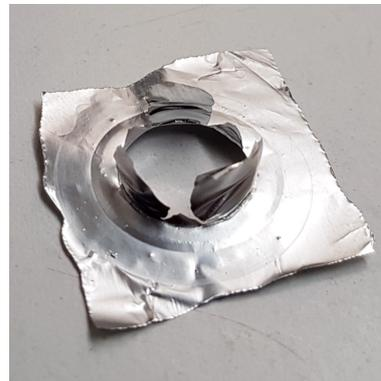
(c) Membrane of aluminum foil after rupture
