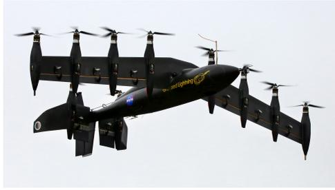
Figure 1.3: NASA GL-10 convertible drone. Source: *www.nasa.gov*
