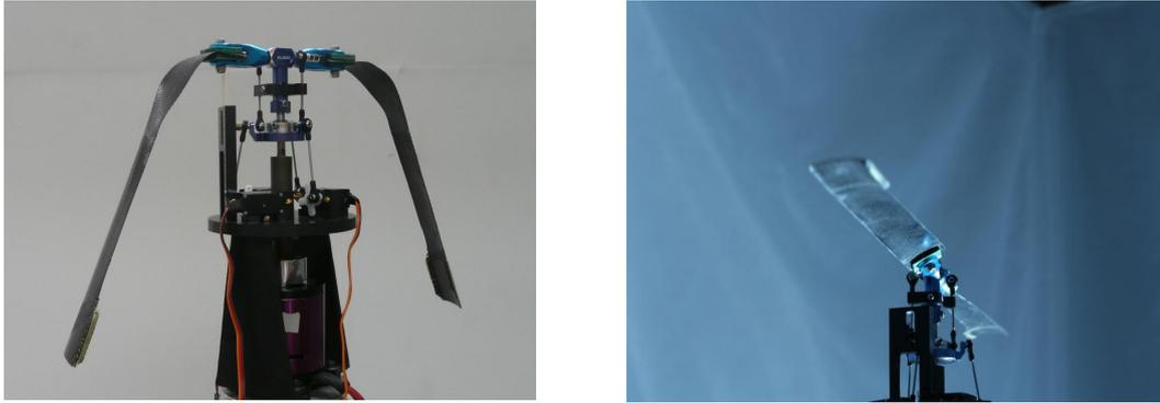
Figure 1.2: Rotor with very flexible blades. Left: at rest; right: rotating. From Sicard (2014).
