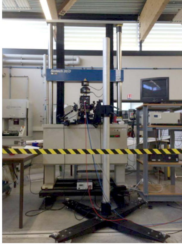
Figure 6.26 – SINTECH 20/D machine used for buckling experiments.
