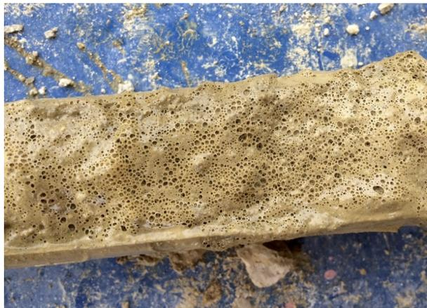
**Figure 9.10:** Soil sampled in the cell three weeks after the injection.
