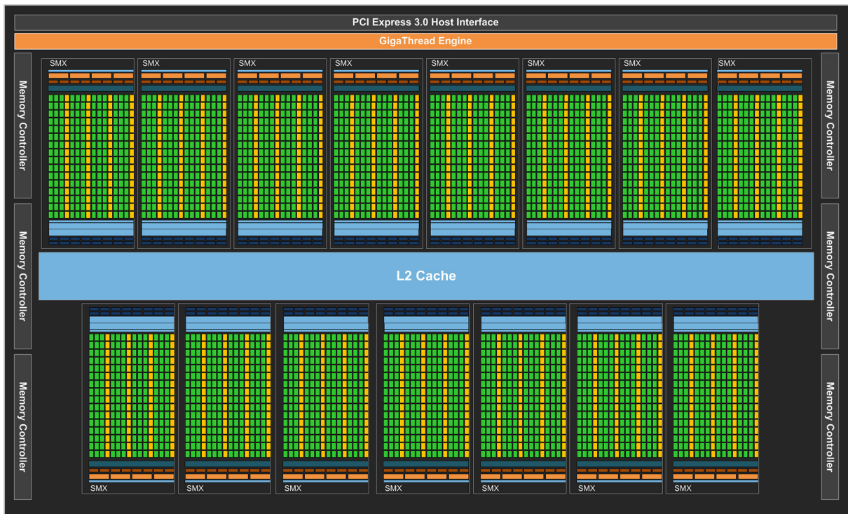
Figure 2.6: NVIDIA Tesla Kepler architecture. Single-precision cores in green and double-precision cores in yellow. Image from NVIDIA white-paper about the Kepler architecture[Nvi12]
