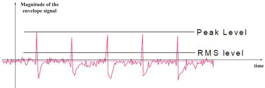
Figure II.3: Crest Factor Representation for Complex Modulated Signal
