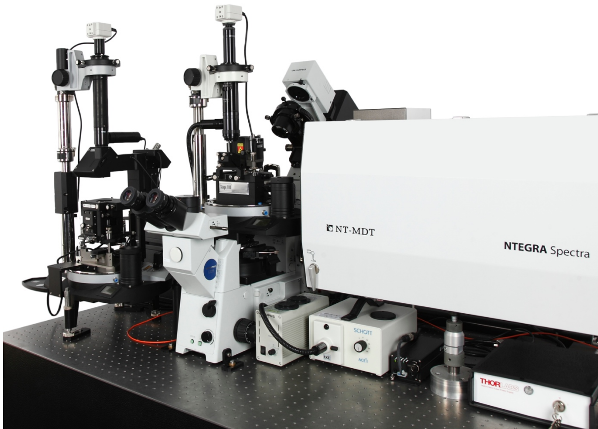
Fig. 2.2 NT-MDT SPECTRA. Atomic force microscope combined with optical confocal spectrometer
