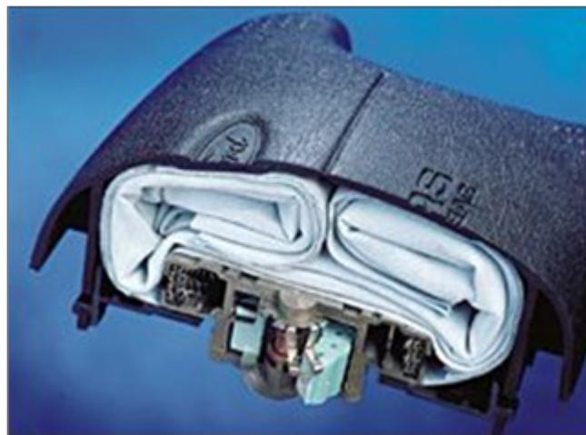
*FIGURE I-21 : PLIAGE DU SAC D'UN AIRBAG CONDUCTEUR - FORD*
