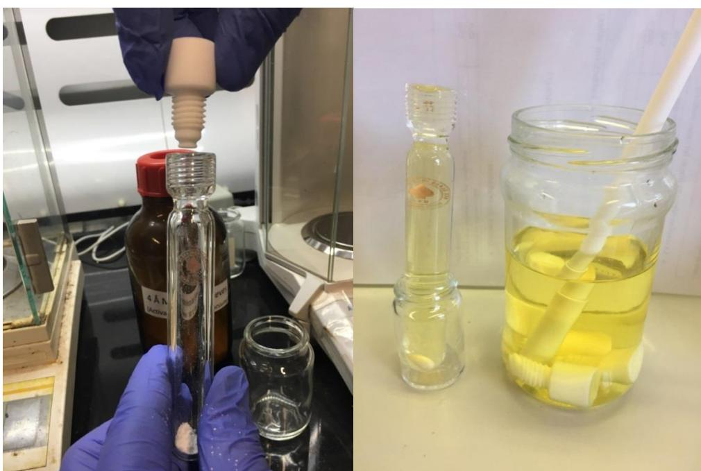
**-HFIP** : HFIP was dried by 2 sequential static drying on 3 Å molecular sieves (20% m/v). Plastic syringes should not be reused when using HFIP.
