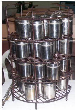
Figure I-13 : Encapsulation du MCP (paraffine) [Pandiyarajan et al., 2011]
