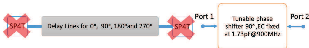
Figure 118: Measurement and simulation condition for tunable phase shifter only
