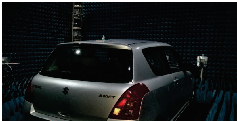
Figure 62: 3D anechoic chamber for the automobile.
