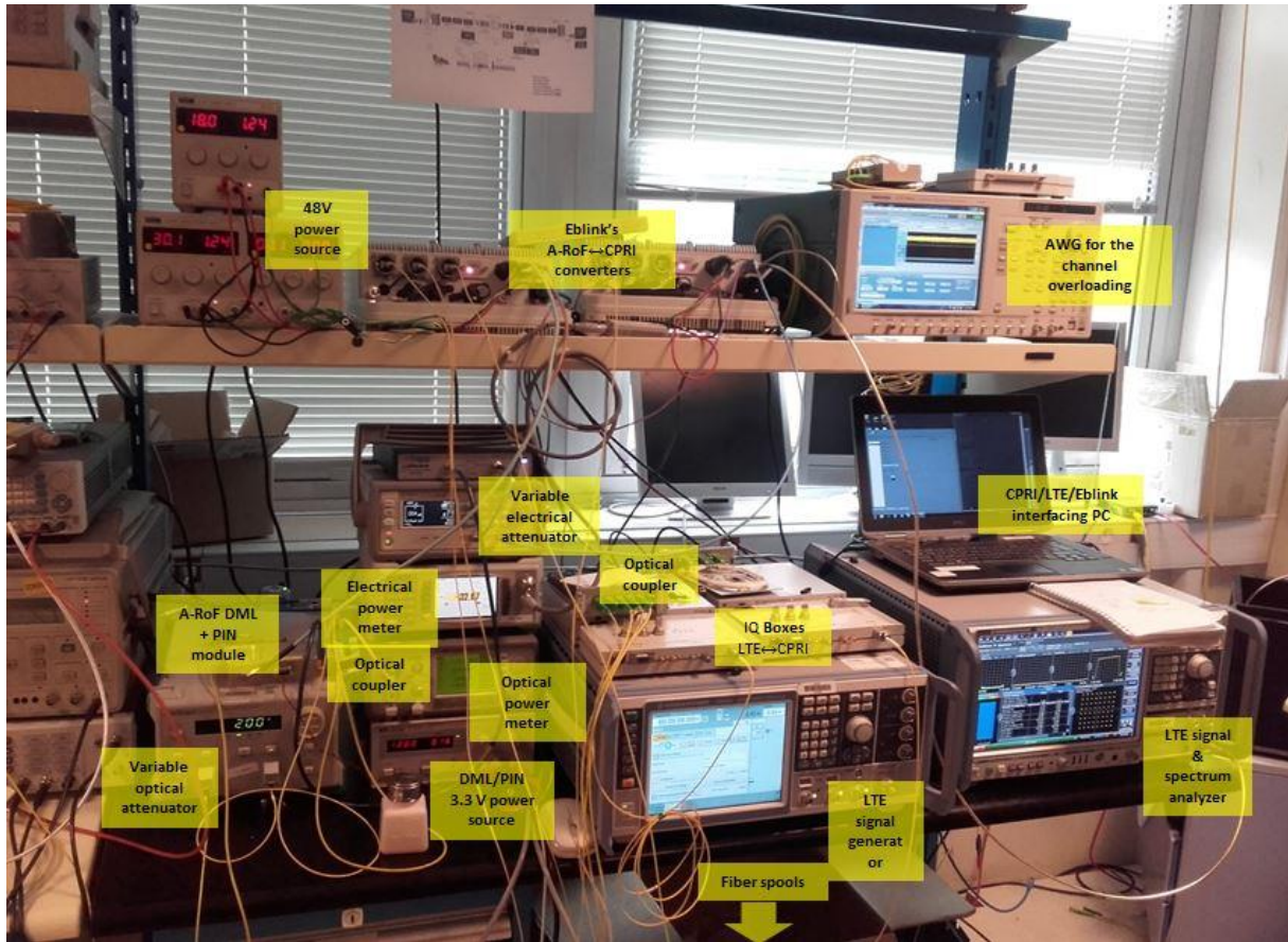
Figure III-4 : A-RoF/D-RoF experimentation (photo)
