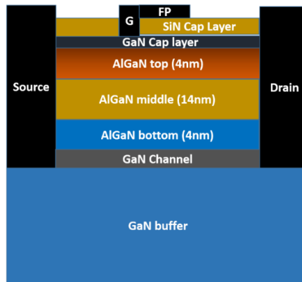
Fig. 3.36. Schematic of the GaN/AlGaIn/GaN HEMT used for transient gate lag simulations.
