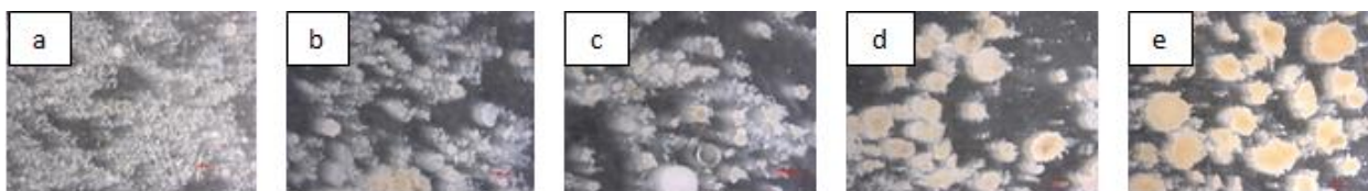
Figure 91: Image analysis photographs of bioflocs/granules of R1 on day [a] 7th day, [b] 14th day, [c] 21th day, [d] 28st day, [e] 42nd day (bar= 500 \mu\text{m} )
