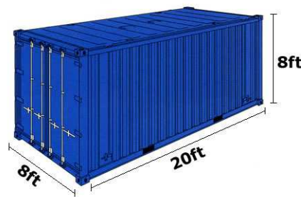
Figure 2.1: Container of 1 TEU. Source: www.dimensionsinfo.com/20ft-container-size/
